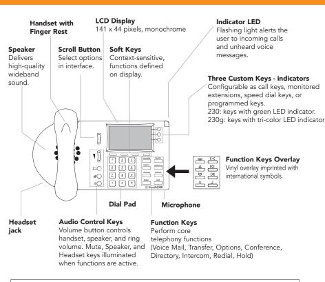
**Note:** You can connect a supported headset into the 230/230g IP Phone by plugging the headset into the headset jack at the left corner of the phone chassis. Contact your system administrator for details.
